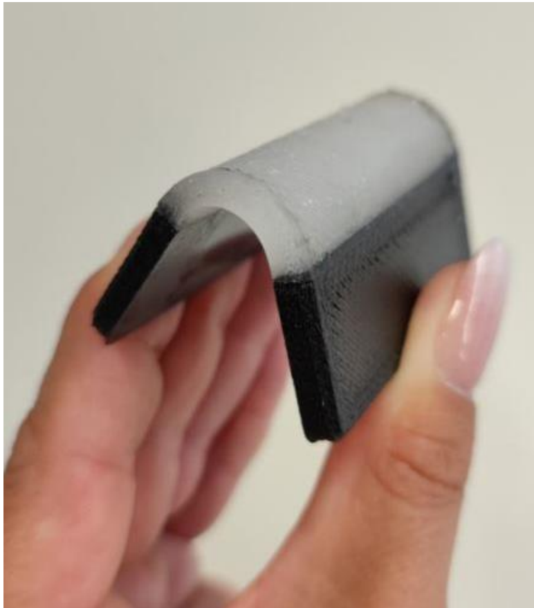
Material: DIPRO®blend H / GF 15 % + DIPRO®flex S60 Source: DIPROmat GmbH
